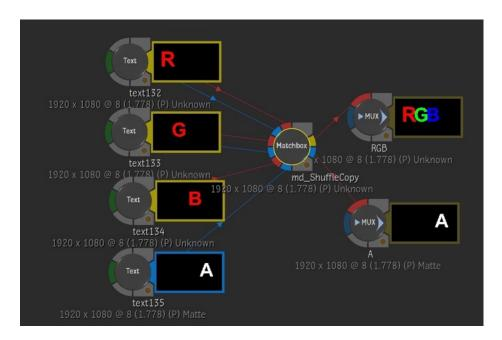
3 front and 3 matte inputs, can be piped into one RGB and one Matte output. This may seem of little use, but I can remember using it a lot in nuke.
