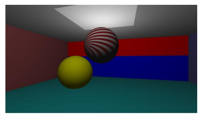
This matchbox adds 2d simulated Global illumination to your 3D scene in action. Using the normals information from the scene, combined with the position data and diffuse information for each pixel, I calculate which pixels would light which pixels and add this light to the scene as in the image below.
