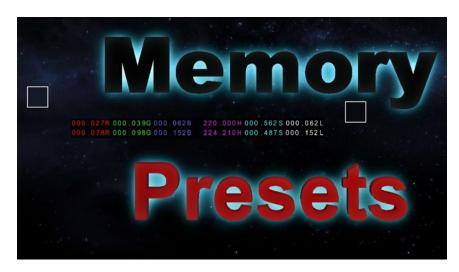
Displays RGB, Hue, Sat and Luminance. You can also enable difference and 2 lines become 1 line Source - Target. If all are zero, then you have a grading match. Use it in context view in batch or as a camera fx in action. Change your color correction upstream and let the numbers guide you to a match.
